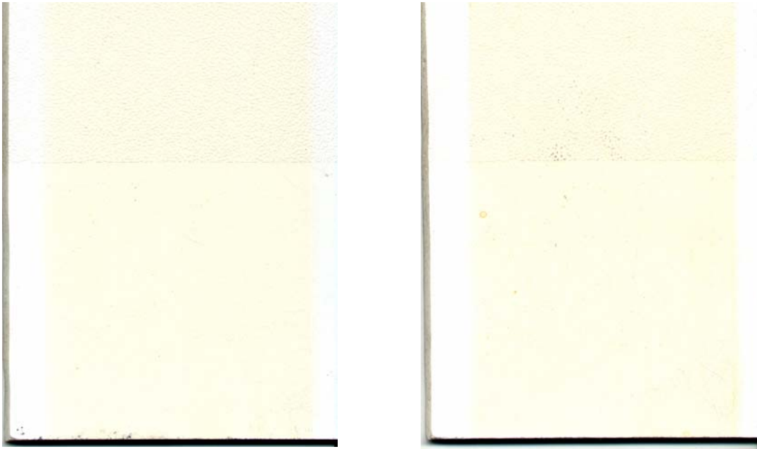
Figure 4. CM-1004 (left) vs. UVS-10287 (right) in System 2; all panels shown as after 2000 hours xenon arc exposure.
