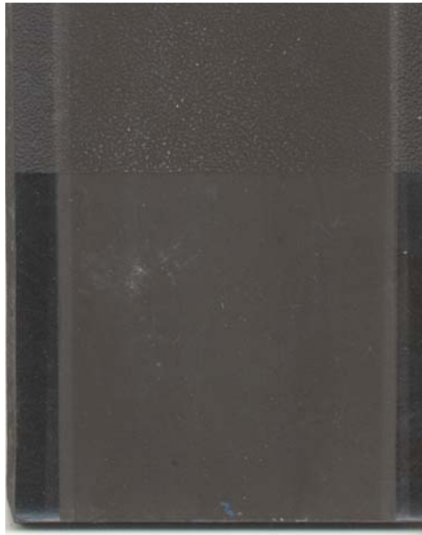
Figure 1. System 1 with 2% Plasticolors CF-20737 at 2000 hours xenon arc exposure.
